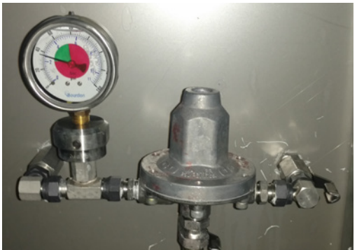
Using Fluid Pressure and Fluid Flowrate control at the Cleaning station:
