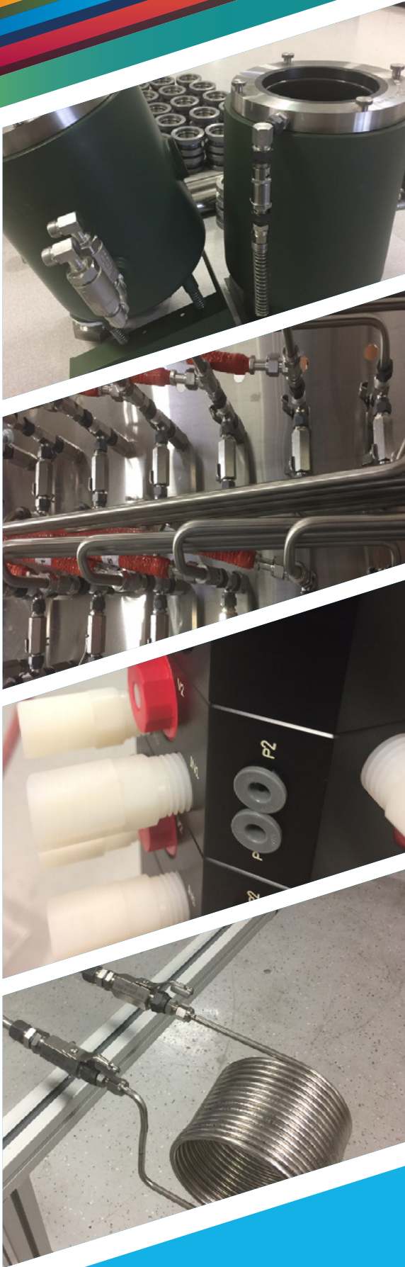
Bell Washer Optimization Project to reduce spray defects from Bell and increase time between housekeeping and service intervals, plus tool free connections for the blow off ring.
