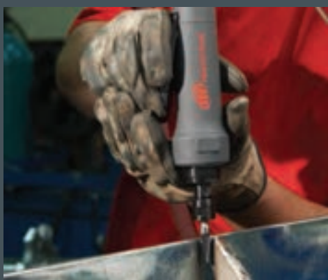
Weld cleaning and smoothing
